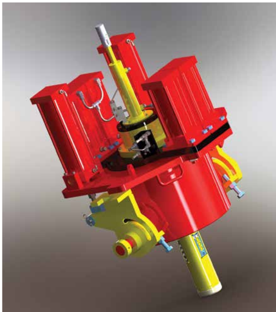
Custom designed motion- compensated ILT for small diameter casing applications
